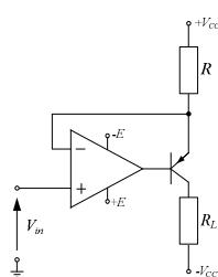
$$I_L = \frac{V_{cc} - V_{in}}{R}$$
