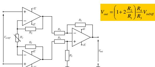
$$V_{out} = \left( 1 + 2 \frac{R_2}{R_1} \right) R_4 V_{inDiff}$$
