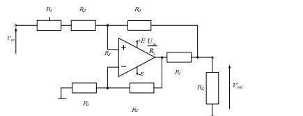
$$I_L = \frac{V_{in}}{R_1} + \frac{R_2 - R_3}{R_1 R_3} V_{out} \Big|_{R_2=R_3} = \frac{V_{in}}{R_1}$$
