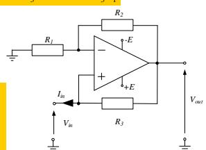
$$R_{in} = -R_3 \frac{R_2}{R_1}$$
