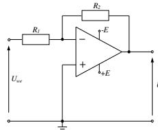
$$A_v = -\frac{R_2}{R_1} \frac{1}{1 + \frac{R_1 + R_2}{A_{v,OL} R_1}} \approx -\frac{R_2}{R_1}$$
