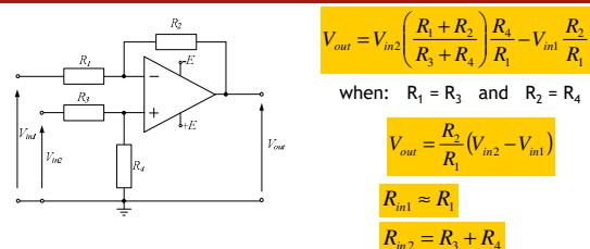
$$V_{out} = V_{in2} \left( \frac{R_1 + R_2}{R_3 + R_4} \right) R_4 - V_{in1} \frac{R_2}{R_1}$$
