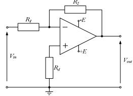
$$R_d = \frac{R_1 R_2}{R_1 + R_2}$$
