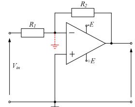
$$I_{in} = \frac{V_{in}}{R_1} \quad I_{out} = \frac{V_{out}}{R_2}$$
