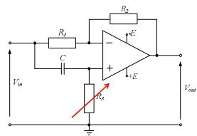
$$\frac{V_{out}}{V_{in}} = -\frac{1-sCR_3}{1+sCR_3}$$
