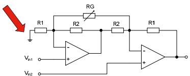
$$V_{out} = (V_{in2} - V_{in1}) \left( 1 + \frac{R_3}{R_2} + \frac{2R_1}{R_G} \right)$$
