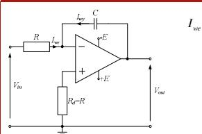
$$I_{we} = \frac{U_{we}(t)}{R} \quad I_{in} = I_C = C \frac{dV_{out}(t)}{dt}$$
