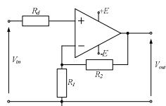
$$A_v = \left( 1 + \frac{R_2}{R_1} \right) \frac{1}{1 + \frac{R_1 + R_2}{A_{v,OL} R_1}} = 1 + \frac{R_2}{R_1}$$
