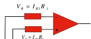
$$V_{out(off)} = (I_B(R + \Delta R) - (I_B + \Delta I_B)R) A_v = \\ = (\Delta I_B R + I_B \Delta R) A_v \underset{\Delta R=0}{\approx} \Delta I_B R A_v$$
