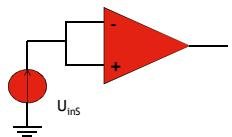
$$V_{OUT} = \frac{A_v}{CMRR[V/V]} V_{inS}$$
