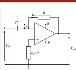
$$I_{in} = C \frac{dV_{in}(t)}{dt} \quad I_{out} = \frac{V_{in}(t)}{R}$$
