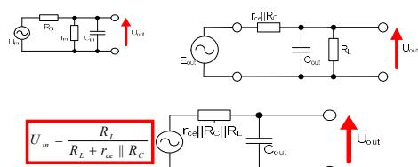
$$f_{2out} = \frac{1}{2\pi(r_{ce} \parallel R_C \parallel R_L)C_{out}} = \frac{1}{2\pi(r_{out} \parallel R_L)C_{out}}$$
