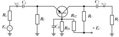
$$f_{2in} = \frac{1}{2\pi(R_G \| R_E \| \frac{r_{be}}{\beta})C_{be}}$$
