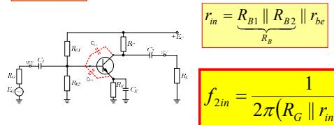
$$r_{in} = \underbrace{R_{B1} \parallel R_{B2}}_{R_B} \parallel r_{be}$$
