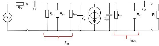
$$f_{2in} = \frac{1}{2\pi(R_G \parallel r_{in})C_{in}}$$
