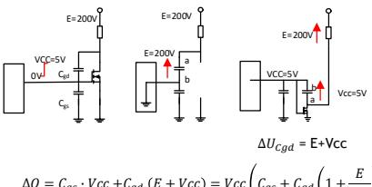
$$\Delta Q = C_{gs} \cdot V_{cc} + C_{gd} (E + V_{cc}) = V_{cc} \left( C_{gs} + C_{gd} \left( 1 + \frac{E}{V_{cc}} \right) \right)$$
