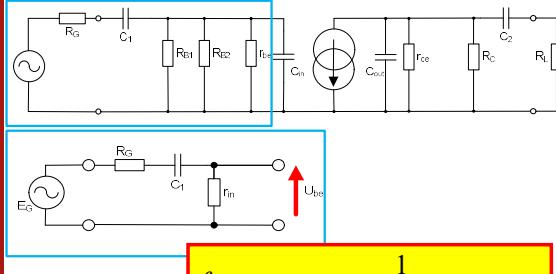
$$f_{1in} = \frac{1}{2\pi(R_G + R_{B1} \parallel R_{B2} \parallel r_{be})C_1}$$
