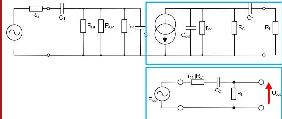
$$f_{1out} = \frac{1}{2\pi(R_C \parallel r_{ce} + R_L)C_2} = \frac{1}{2\pi(r_{outCE} + R_L)C_2}$$
