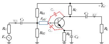
$$f_{2in} = \frac{1}{2\pi((R_G \parallel R_B + r_{bb'}) \parallel r_{be})C_{in}}$$
