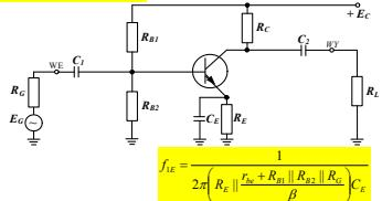
$$f_{1E} = \frac{1}{2\pi \left( R_E \parallel \frac{r_{be} + R_{B1} \parallel R_{B2} \parallel R_G}{\beta} \right) C_E}$$
