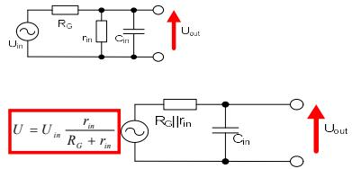
$$f_{2in} = \frac{1}{2\pi(R_G \parallel r_{in})C_{in}}$$
