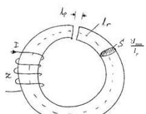
$B_{\max} = 0.05 \dots 0.1 \dots 0.2 \dots 0.3$  [T] for ferrites
