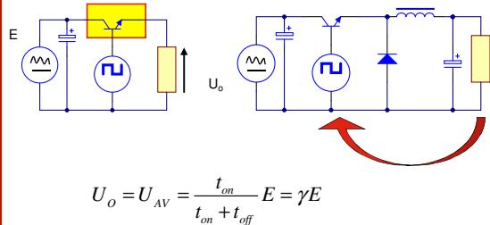
$$U_o = U_{AV} = \frac{t_{on}}{t_{on} + t_{off}} E = \gamma E$$
