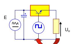
$$U_o = U_{AV} = \frac{t_{on}}{t_{on} + t_{off}} E$$
