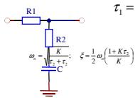
$$\tau_1 = R_1 C \quad \tau_2 = R_2 C \quad K = k_d k_f$$
