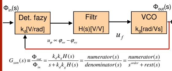
$$G_{zam}(s) \equiv \frac{\Phi_{out}}{\Phi_{in}} = \frac{k_d k_g H(s)}{s + k_d k_g H(s)} = \frac{\text{numerator}(s)}{\text{denominator}(s)} = \frac{\text{numerator}(s)}{s^{\text{order}} + \text{rest}(s)}$$
