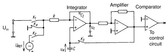
1. For K4 and K3 on, the capacitor C is charged to a voltage  $U_k$  equal to the integrator offset.
